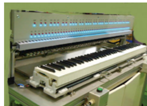
Automated sound quality tester on the piano keyboard production line
