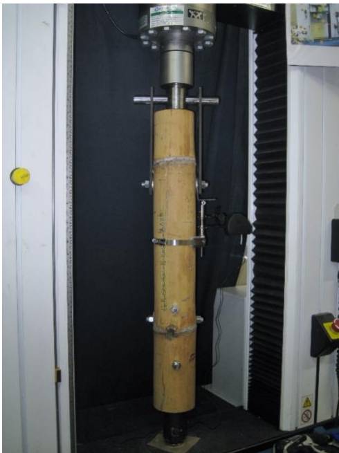
Figure 5. Tests of physical and mechanical properties of the Mexican guaduas
