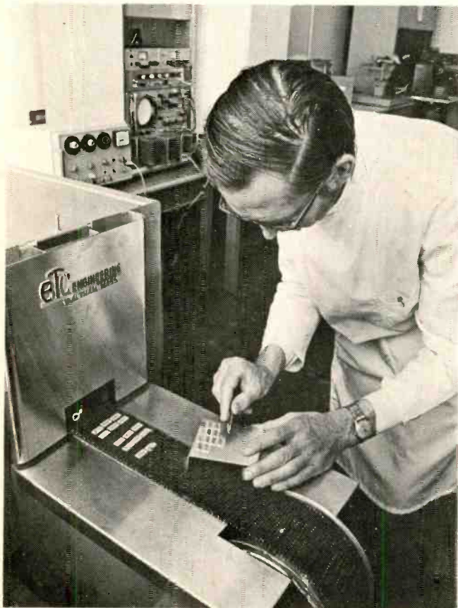
Loading printed substrates into a belt furnace. Photo courtesy Middlesex Polytechnic.
