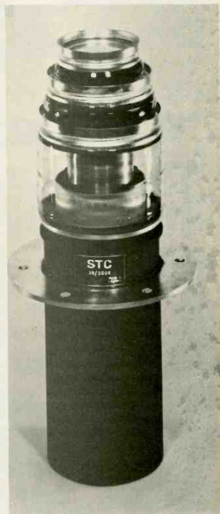
Industrial heating triode with integral water jacket. Filament 8V, 300A; Anode 13K Vmax, 10A max.
