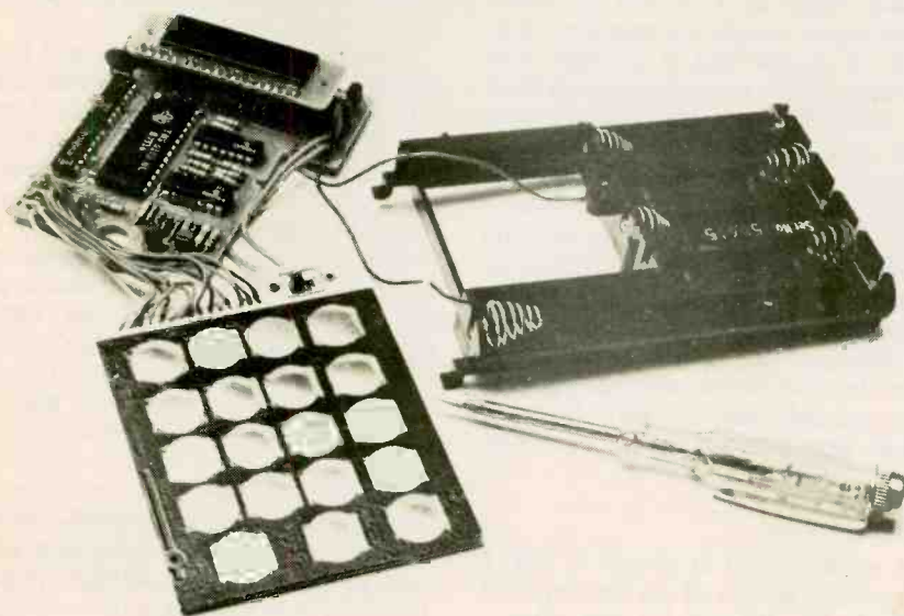
The main circuit board, the key board and the battery holder of the kit built by ETI.
