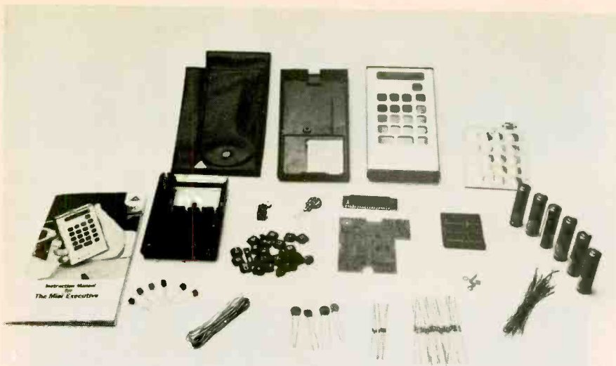
As the photograph shows, there are relatively few components to the Advance International Calculator kit. It can be built in under three hours.
