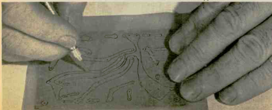
Fig. 7. Remove the unwanted film, leaving film over the areas where copper is to remain.
