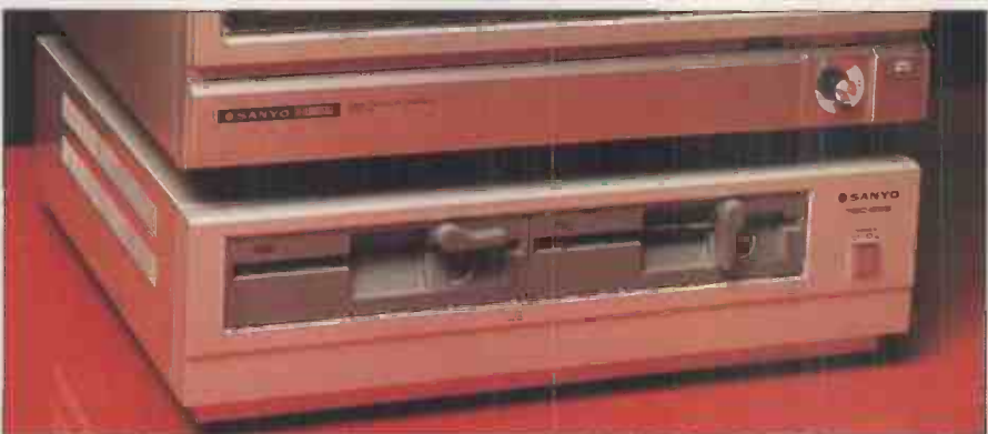
The two 360k disk drives are double-sided and the locking lever is easy to use
