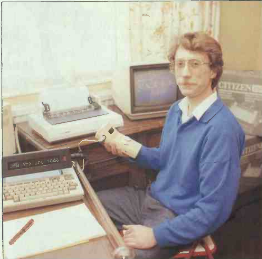
Developed by the Royal National Institute for the Blind and produced by Dolphin Systems, the battery-powered Mimic speech synthesiser is ideal for use with the NEC laptop, the BBC Micro and PC-compatibles
