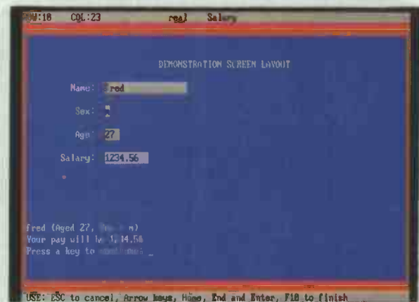
'Option(3)' in the 'option' clause uses Turbo Prolog's built-in 'consult' predicate to access a file which contains information on the screen layout to be used
