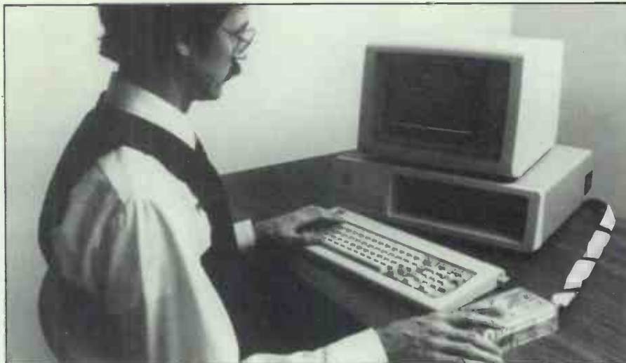
This Braille Screen Reader from IBM combines a mouse with a single Braille cell mounted into its top surface, all in a self-contained unit
