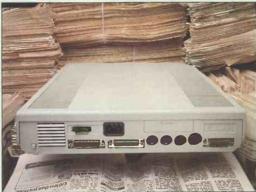
The Mega ST4 contains a very comprehensive collection of ports compared to the 1040ST — the only difference is the addition of a fan
