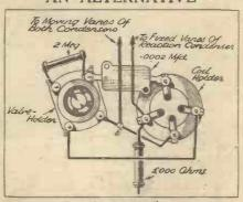
In response to many requests, W. L. S. gives in this diagram the connections for B.T.S. coils in the "Simplex" Two.
