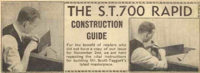
Fig. 1. Here the right-hand side-piece of the cabinet and the top-piece are being fitted together.
