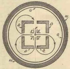
Fig. 5.—In this form of Renode valve the total length of the electron path is deliberately designed to be as long as possible.
