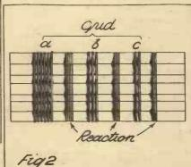
rice 1 shows a suitable coil-switching scheme for short-wave broadcast reception, and Fig. 2 the practical form which the coil should take.
