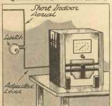
A switch arranged as seen here will save much twiddling of the volume-control knob.
