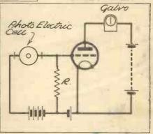
A simple use of the photo-electric cell to give a visual indication of change in light intensity.
