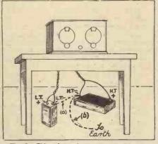
Fig. 3.—This scheme is a very common one, many short-wave enthusiasts placing their batteries on the floor beneath the set as shown.
