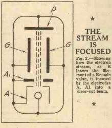
In order to make this method of control more effective, the electrons as they leave the filaments are first concentrated into a beam, so that in this respect the new valve rather resembles a cathode-ray tube.
