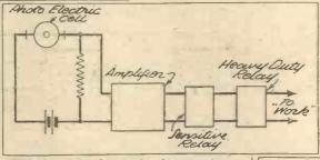
With this chain of apparatus, lamps, motors, bells, etc., can be controlled by a beam of light.
