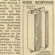
This is a drawing of the latest ribbon microphone which introduces very little frequency distortion.
