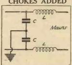
Fig. 2. This circuit is useful in cases of high-impedance electrical plant.
