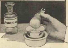
A layer of wax, a coarse needle, some fluorspar and sulphuric acid are all that you need.
