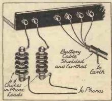
Fig. 4.—In this case the battery leads are taken through a shielded cable, the shield being earthed.
