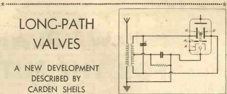
Fig. 3.—When the signals are applied across the grid wires G, the electron stream will be deflected first to one grid and then to the other.
