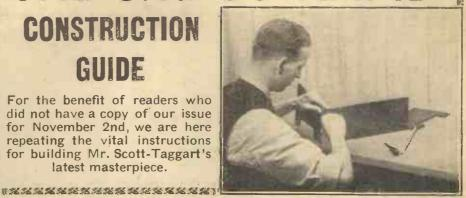
Fig. 2. The first stage in assembling the "Easy-Cabinet." Fixing the left-hand side-piece to the top.
