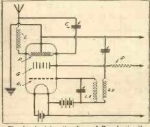
Fig. 4.—An interesting form of Renode circuit. Magnetic and electrostatic control are both used in this scheme.
