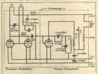
The screening in this experimental circuit need not be elaborate, couple of inverted biscuit tins will probably be quite sufficient.
