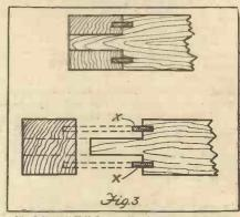
The letters "X" denote the feather slips in this diagram of a mortised and tenoned joint.
