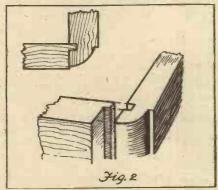
Fixing a panel by means of a rebate in the cabinet
