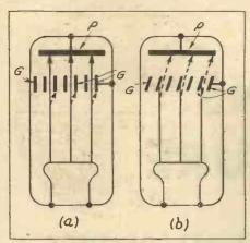
Fig. 1.—Controlling the electron stream by deflection. In (a) the grid wires G are set parallel to the path of the stream. In (b) the wires G, instead of being arranged parallel to the stream, are inclined to it.
