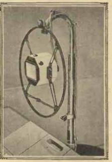
The carbon microphone is the oldest type still in use. It takes the form nowadays of the Marconi-Reisz instrument, which is a form of transverse current microphone. A rectangular recess about 1-16th inch deep is made in a block of marble and a carbon electrode is sunk in the block at each end of the recess, which is next covered by a mica diaphragm.
