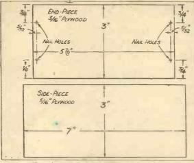
Two pieces of wood of each of the above sizes are required to carry the Triple Extractor panel.
