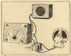
When an extension speaker is directly connected to the output terminals of the S.T.700 two condensers should be interposed to prevent H.T. being fed through the extension wires.
