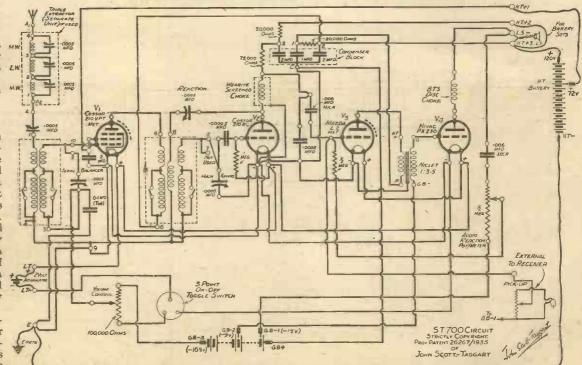
The circuit of the famous S.T.700, showing how the Triple Extractor is connected, and the use of a pick-up for gramophone work.
