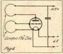
An interesting experiment consists of seeing whether you can make your set oscillate with a 1½-inch turn of wire in place of each coil.
