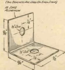
The two outside diagrams (Fig. 11, left, and Fig. 13, right) show how the terminal strips are drilled, while the centre sketch (Fig. 12) depicts one of the brackets used in the set, two for each strip.
