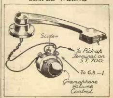
How a pick-up and external volume control are connected to the S.T.700.
