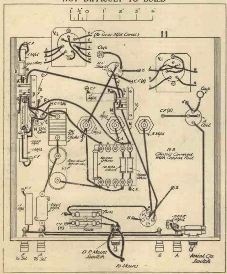
The great majority of the wiring is carried out on the under-side of the chassis, which is made of plywood covered with metal foil.
