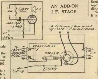
A simple resistance-capacity amplifier particularly suitable for addition to the "Simplex" Two.
