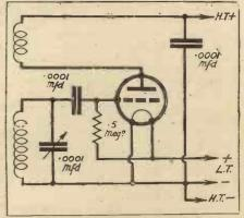
Fig. 2.—The circuit is really that of an ordinary oscillating detector minus its reaction control.
