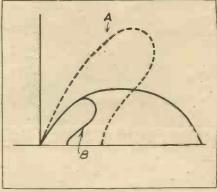
Fig. 4. Here we see how the sky-wave (A) is radiated at night for the benefit of distant listeners, and how in the daytime the normal sky-wave B is completely suppressed, the energy being added to the ground-wave, shown as a solid line.
