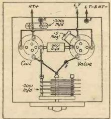
Fig. 1.—The layout of the calibrated oscillator described by W. L. S. The wavemeter is housed in a simple aluminium box.
