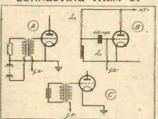
Three methods of coupling microphones. A is the carbon type, B the condenser, and C the moving-coil variety.
