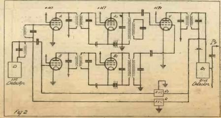
This is a scheme for combining A.V.C. with selectivity control, so that the set automatically adjusts itself both as regards sensitivity and selectivity under all conditions.
