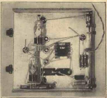
The Cossor valves are here shown in position under the baseboard. The heptode is the lower one and the screen pentode is above it.
