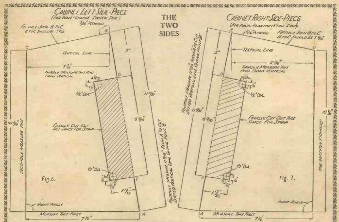
The sides of the cabinet should be cut out in the manner shown. The 1-in. diameter holes are to allow the saw to complete the cutting of the space for the terminal strips. If wood surfaces are polished lines marked "vertical line" should be drawn on paper affixed to the wood.
