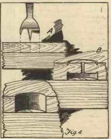
Cutting a hole in a piece of wood in order to prevent breaking through on the reverse side.
