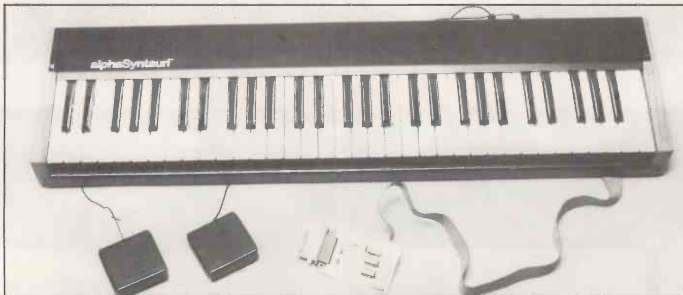
A five-octave keyboard with velocity-sensitive keys puts Alpha Syntauri top of the line for digital synthesis.
