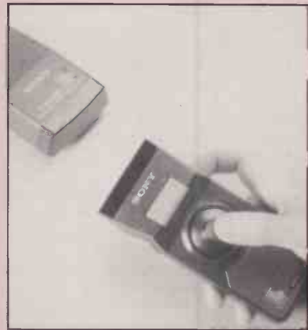
An infrared sensor attaches to the computer so that you can use the joystick from across the room.
