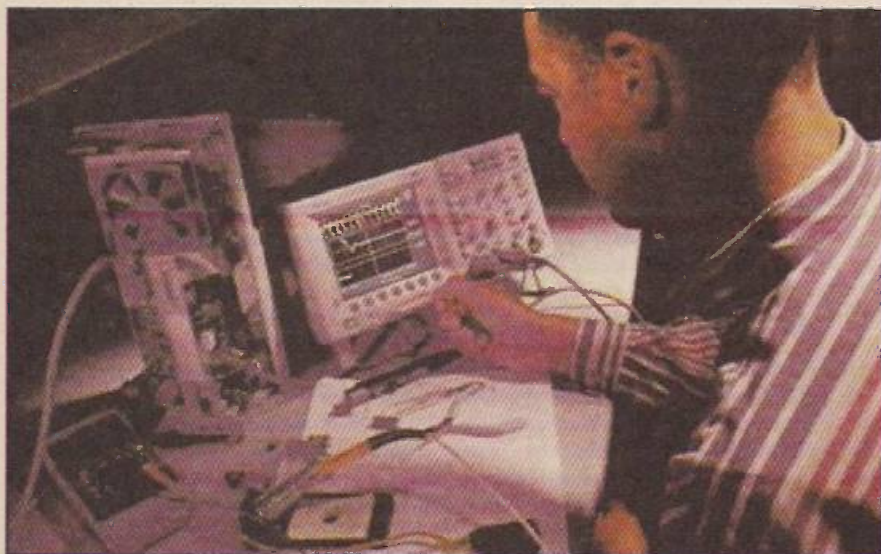
The Tektronix TDS3054B four-channel digital phosphor oscilloscope has a bandwidth of 500MHz and a sampling rate of 5GS/sec per channel.
