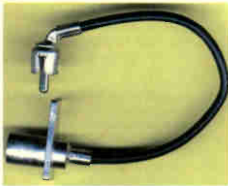
Photo 2: RF output connector for the Panasonic TU-DSB31 digibox.
