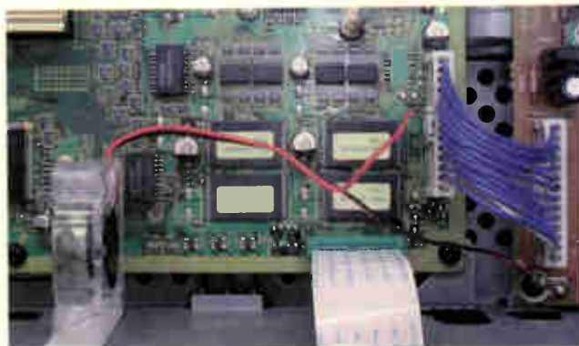
Photo 1: Multi-pin connectors between the power supply and main PCB in the Panasonic TU-DSB30 digibox. Also, the addition of a miniature cooling fan to remove 'hot spots'.
