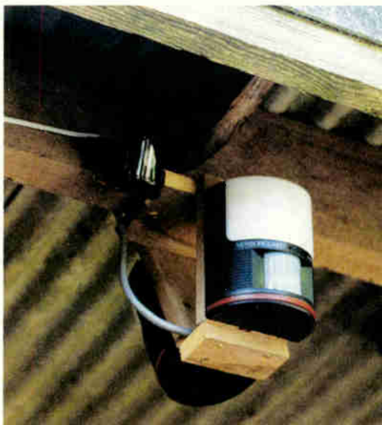
Sensor based on a modified Sensorguard battery-operated lamp.
