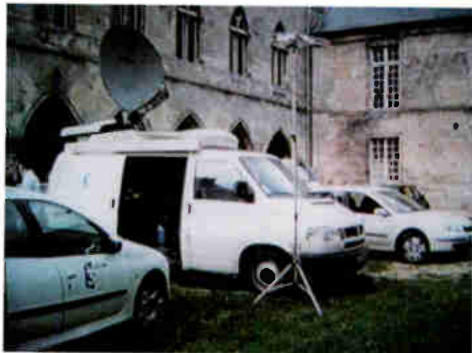
A French satellite uplink truck at an OB location. The active caravan aerial on the small mast is used for terrestrial off-air cueing purposes.
