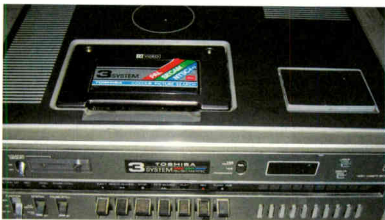
Photo 8: Toshiba Beta machines are relatively uncommon today. This Model V5480 has been retained because of its multi-standard operation.
