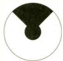
Fig. 3: The magic-eye display.
