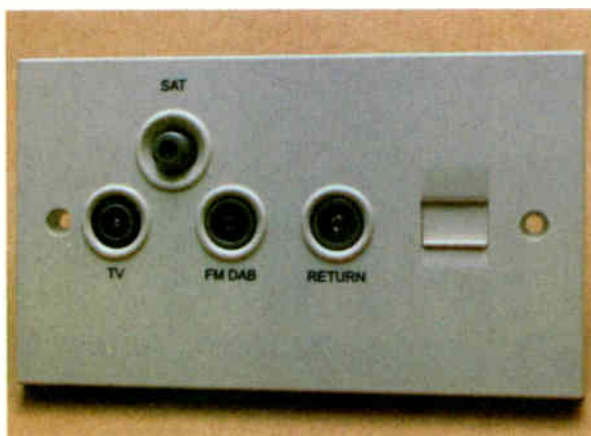
Figure 9: The Labgear PSW242T, which is typical of the various makes of 'master' wallplate, includes a triplexed satellite/UHF/VHF outlet, a socket for the main return feed to other rooms and a phone socket.
