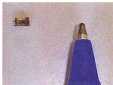
Comparison of the tiny inverter-PCB fuse with the tip of a ball-point pen.
