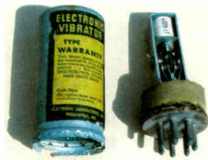
Photo 2: Our thanks to Roger Goodman who provided this picture of a car radio vibrator unit.
