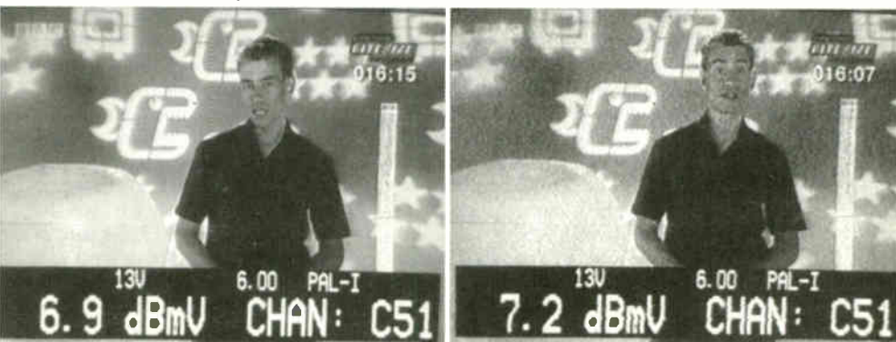
Figure 8: The effect of LNB noise on UHF analogue reception. These shots are from the same installation as the spectrum-analyser displays in Fig. 5. Note that although the signal level remains about the same the picture on the right (with the LNB connected to the multiswitch) is very snowy.
