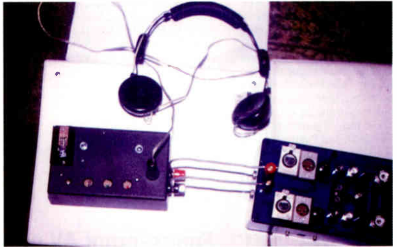
Photo 1: The cable tester (left) and cable box (right) with headphones ready for use. The 'portholes' in the tester are for the LEDs and lamp. The BD238 shunt-regulator transistor and its heatsink are mounted on the case at the top left.
