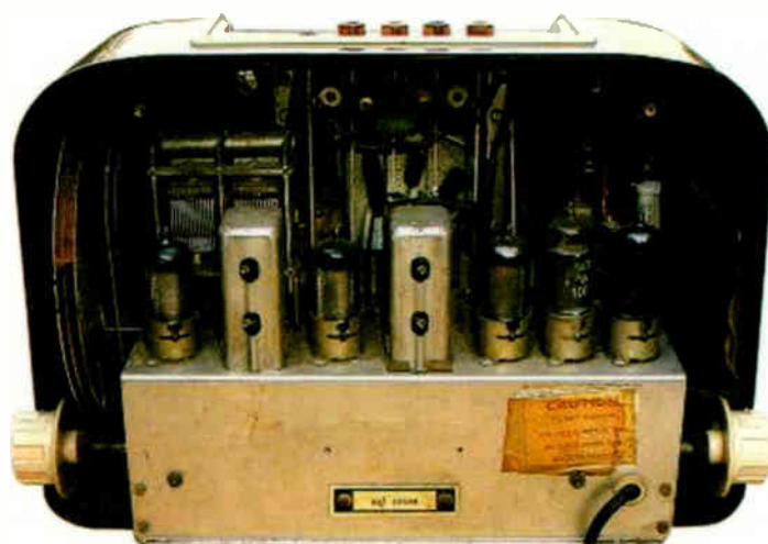
Rear view of the Bush Model DAC10 with the back cover removed.
