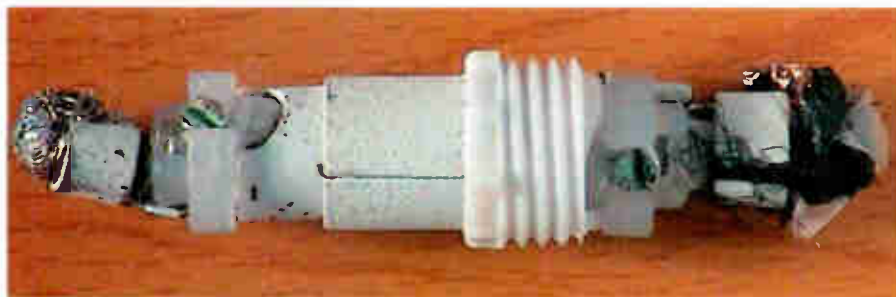
Photo 1: Cable 'join' damaged during building work.
