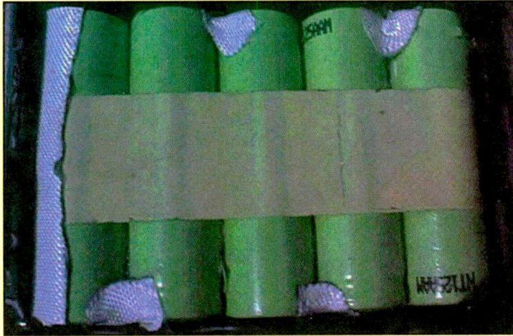
Fig. 3: Extra insulation (glass fibre tape) added in a mobile phone battery pack.
