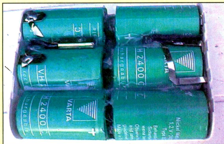
Fig. 4: Laptop battery pack rebuilt using NiMH cells.
