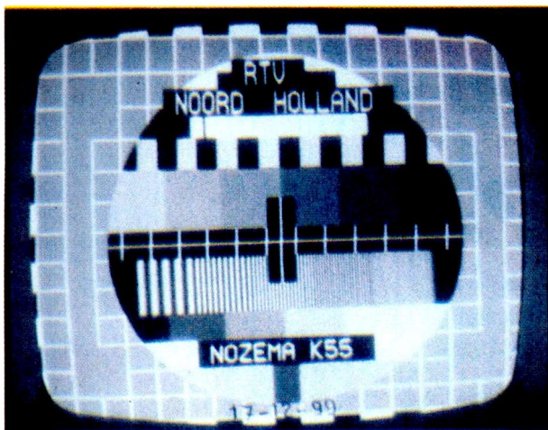
PM5544 test pattern transmitted by the RTV Noord Holland station at Wormer, on ch. E55. Photo courtesy Ryn Muntjewerff, Holland.
