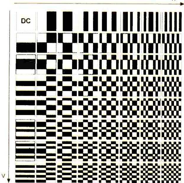
Fig. 7: The 8 x 8 DCT block.
