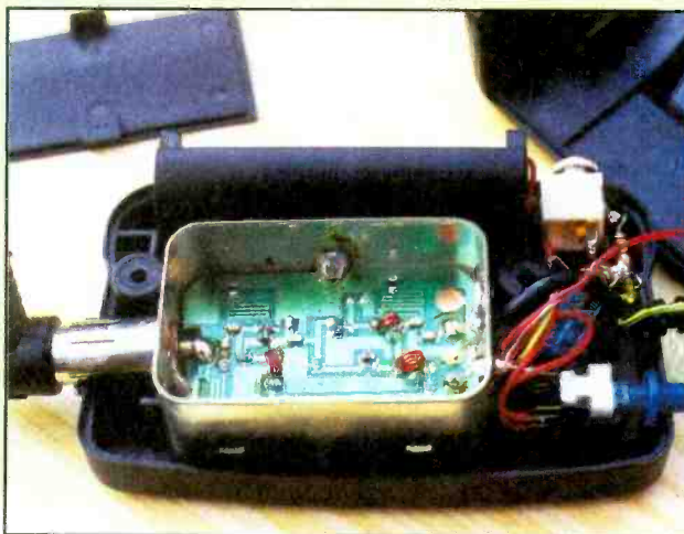
Internal view of the Maplin 6431 two-stage UHF amplifier.
