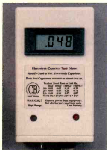
Fig. 1. Prototype \tan\delta meter, measuring a 'good' board-mounted electrolytic.
