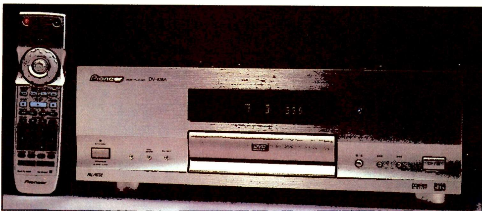
The Pioneer DV-828A DVD-Audio player can handle a recorded bandwidth greater than 20kHz.
