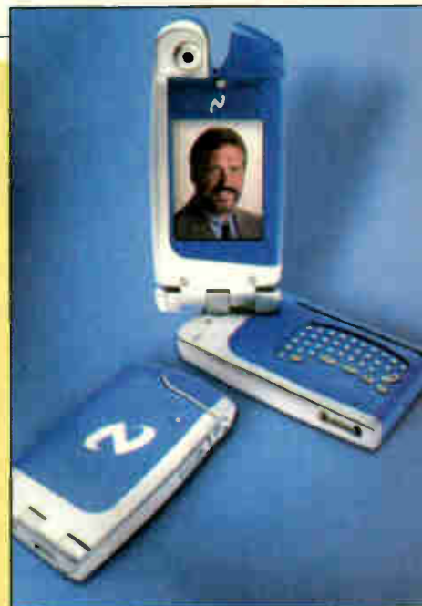
National Semiconductor has unveiled a prototype hand-held device, the Geode Origami, that combines eight consumer electronic products in one unit. It's the size and weight of a small digital camcorder and folds and unfolds to provide the various functions – wireless video communication and phone, digital camera, camcorder, MP3 audio player, PDA, internet access and e-mailing. It uses Microsoft Windows OS software.
