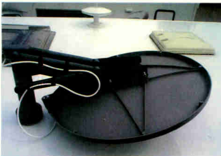
Photo 4: Cable loops arranged to allow free movement of the dish.
