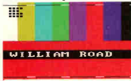
Photo 3: As Photo 2 but note different missing square in block at top left.
