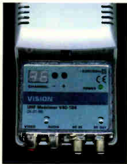
The V40-104 UHF modulator from SatCure with integral power supply (top). For full information go to http://www.satcure.com
