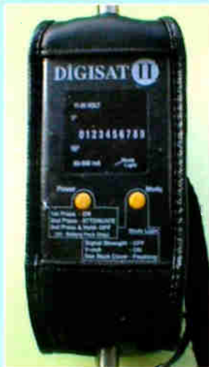
This digital satellite meter – namely Digimeter – is designed to simplify dish installation. (Picture courtesy Digital Sales)
