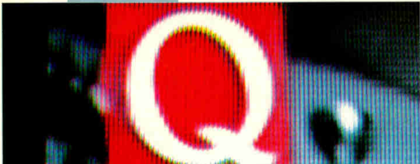
The type of logo that can cause phosphor burn. This one is for the Q network
