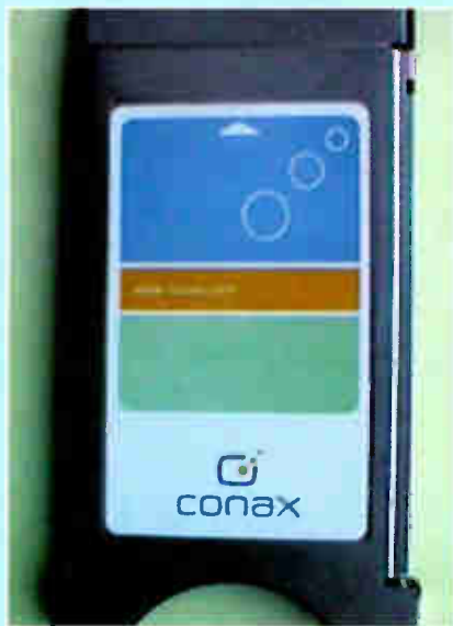
Module for inside a receiver allowing decryption of Conax channels – with appropriate card inserted. (Picture courtesy Digital Sales)
