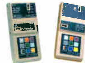
MC 377+ Analogue & Digital, Satellite & Terrestrial Measures channel power and C/N
