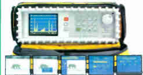
PROLINK 3 SERIES Satellite & Terrestrial, Analogue & Digital, Spectrum Analyser with Optional BER
