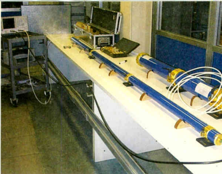
Photo 2: Laboratory test rig for measuring the screening factor.
