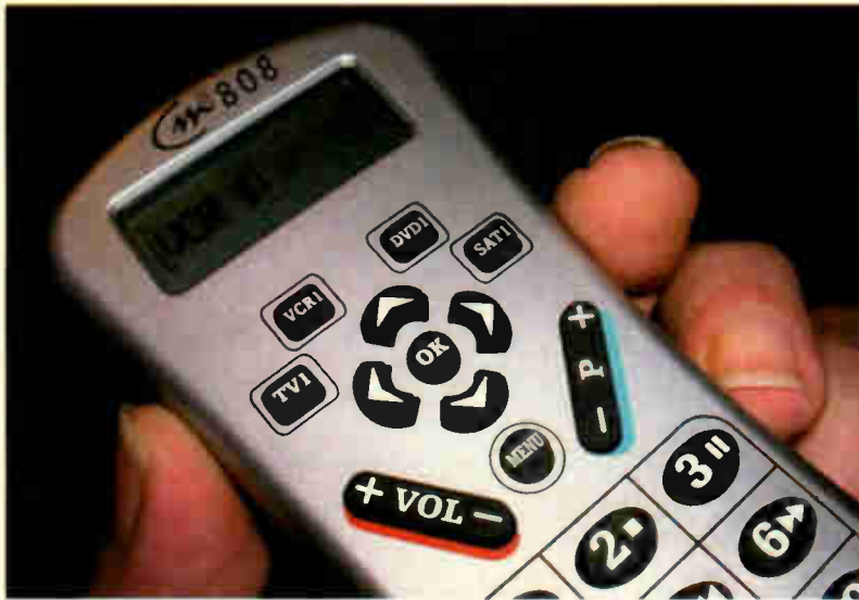
Photo 3: The CM808 universal remote-control handset from Wallis Universal. Note the LCD programme indicator.
