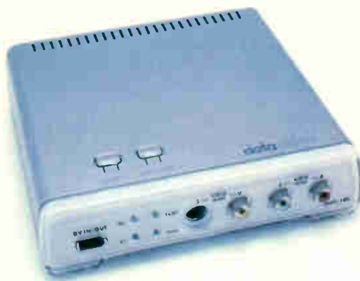
Photo 7: This unit from Datavision can program a camcorder for DV in by rewriting its software.
