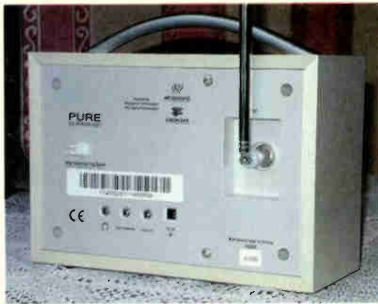
Photo 2: The rear-panel connections to the Evoke-1 DAB receiver.
