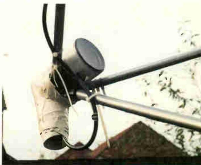
A washing-up liquid plastic bottle, with gaffer tape, can be fashioned to provide a protective cover for your LNB. Apply white spray paint to improve the appearance.
