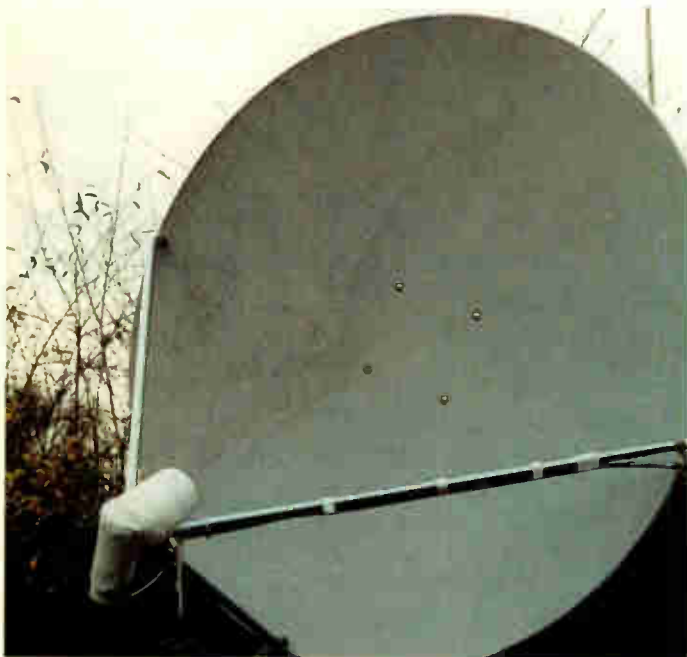
A nice clean dish (right-hand side) – the initial results of my dish cleaning with Somerfield's All Purpose Cleaner. Grime has been left on the left-hand side of the dish to show the effectiveness of the cleaner.
