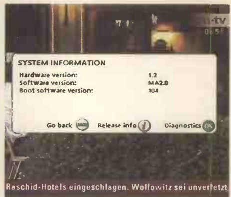
Photo 1: Nokia 9800 receiver software version display.
