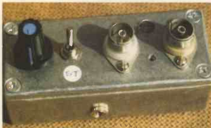
External view of the prototype HS Publications varicap-tuned notch filter for Band I.
