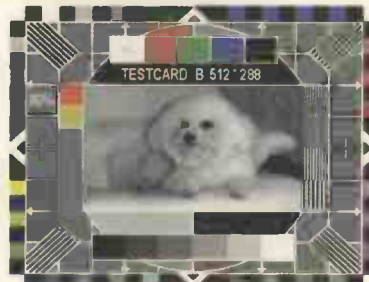
Photo 5: The 4:3 aspect-ratio test pattern B.
