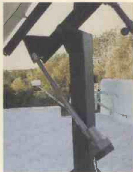
Photo 2: Dish actuator used by Hugh Cocks with his 2m dish's polar mount for satellite tracking.
