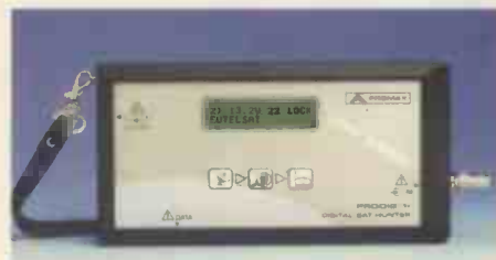
The Prodig 1 digital Satellite Hunter from Promax
