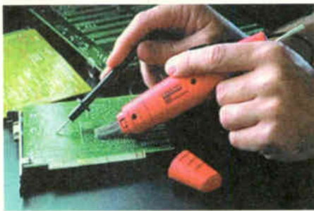
Above: PCB testing with a conductive brush and probe.
