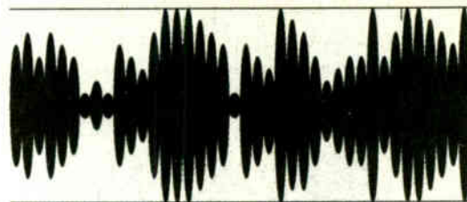
Fig. 5: Representation of variable-area optical sound film recording.
