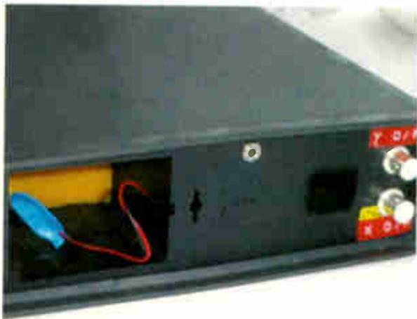
Addition of Y and X output BNC sockets at the rear of the Sadelta meter.
