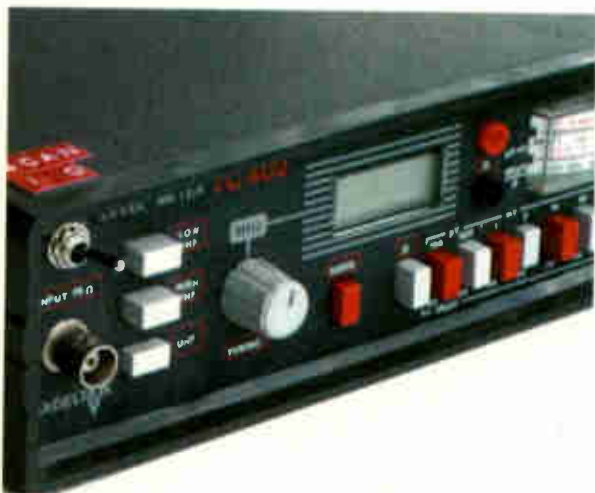
Front view of the Sadelta TC402 signal-level meter with the normal/sweep changeover switch added at the op left of the panel.
