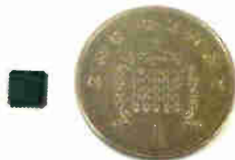
Fig. 1: A CX22496 line-interface chip beside a one-penny piece for size comparison. The chip measures 5mm square, has 28 pins and is housed in a QFN package.
