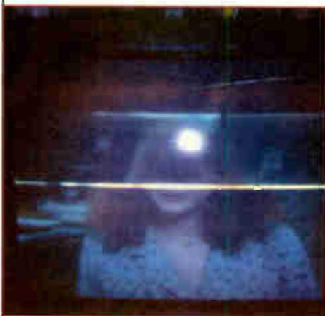
Photo 1: Strange field-scan fault symptom encountered with a Sharp Model 51DT25H.
