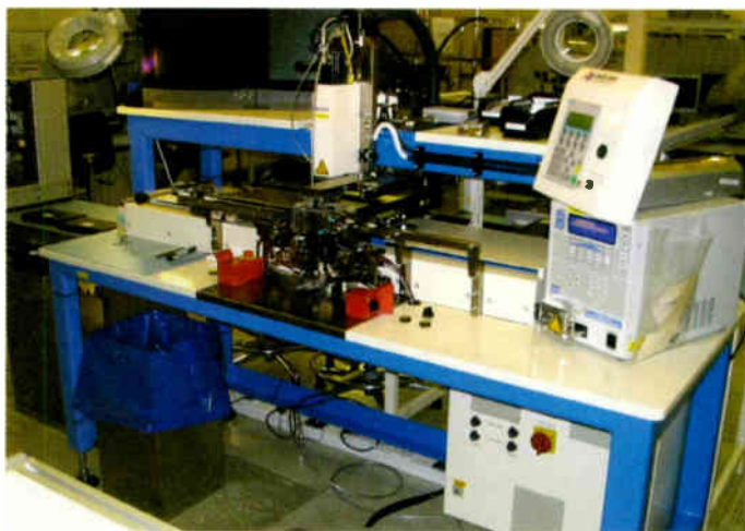
Photo 9 – right: The head of the tab bonder, ready to bond when the new tab is placed in position.
