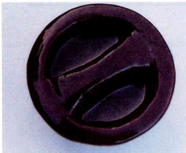
Photo 4: The new wavechange switch knob when painted.
