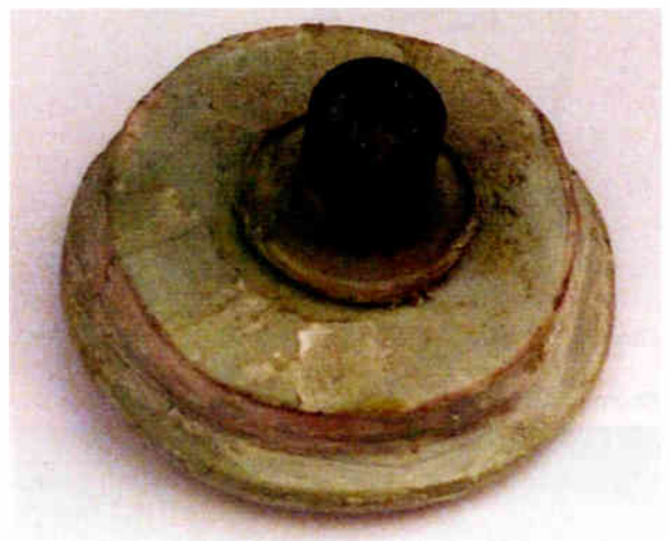
Photo 1: Shaft attached to the moulding for the new wavechange switch knob.
