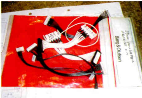
Service Kit 6276331 for checking the boards.
