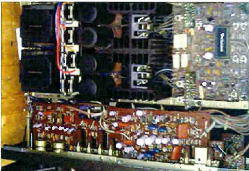
Inside the Technics SU8080 amplifier.
