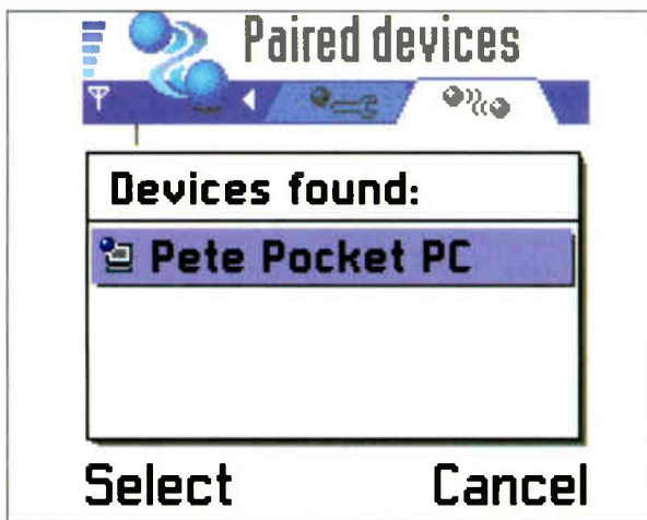
Fig. 6: Typical response to a Bluetooth 'inquiry', showing paired devices.
