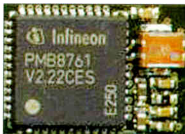
Fig. 1: A typical Bluetooth hardware implementation, by Infineon. Size is 10.6 x 7.3mm.
