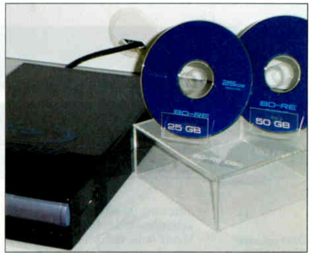
The BD-RE (rewritable) disc is now at version 2.0, while the BD-R (recordable) and BD-ROM (read only) are at version 1.0.
