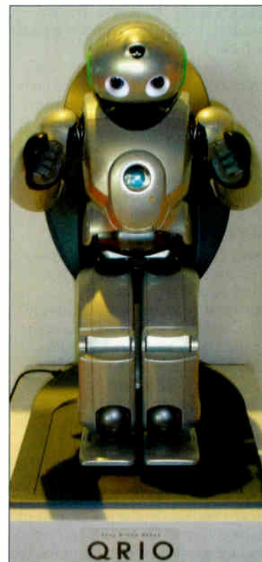
The QR10 Dream Robot is described as the world's most sophisticated humanoid, using voice and face recognition technologies. It can also walk and dance on two legs.
