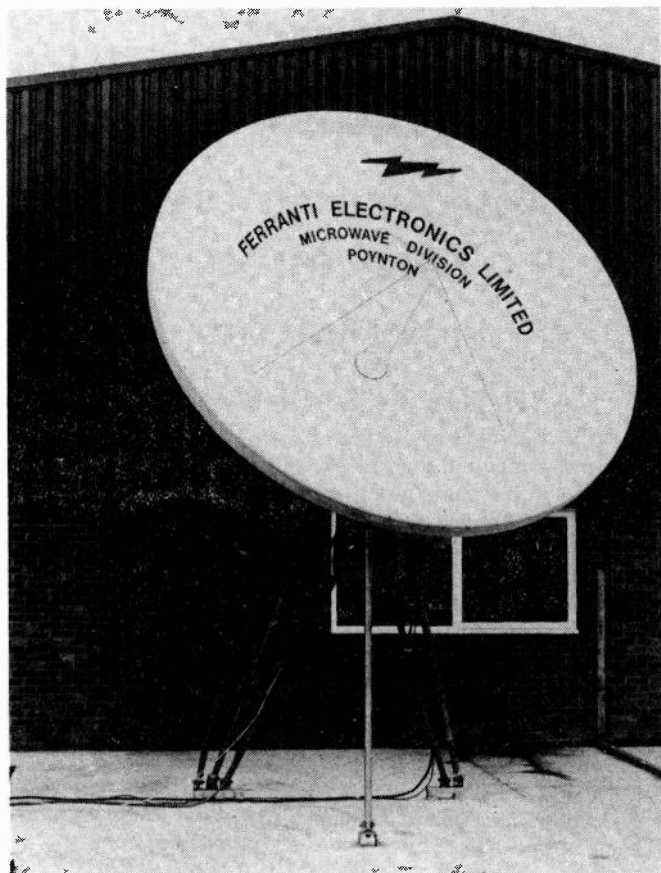
The aerial end of the Ferranti 11.45-11.8GHz satellite receiving system. Dish diameter 3 metres, gain 48.6dBi, with switchable dual linear polarisation.
