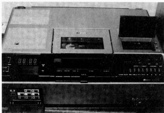
General view of the Sony Betamax VCR. Note timer setting switches on the left and tuning controls under flap at right.
