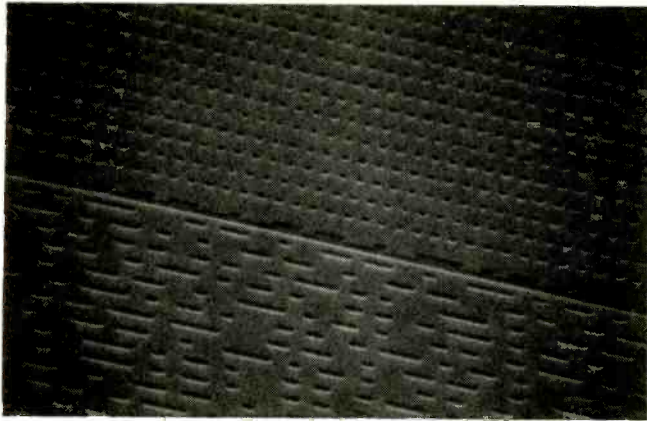
Fig. 6: Scanning electron microscope picture (magnification 2,500 times) showing the transition between the audio and video (smaller pits) sections of a 5in. CDV disc.
