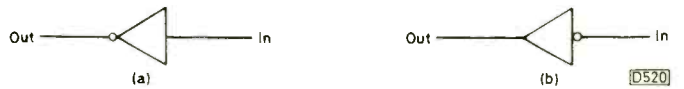
Fig. 4: Symbols used to denote digital transistors. (a) NPN type with type number starting DTC. (b) PNP type with type number starting DTA.
