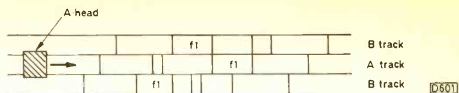
Fig. 16: A DAT head straddles three adjacent tracks.
