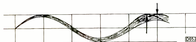
Fig. 3: Tune T2 to equalise the peaks then reset RV1 to restore the signal amplitude.
