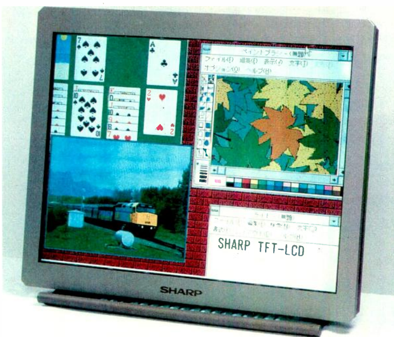
The World's largest direct-viewing TFT LCD display at 28 inches.
