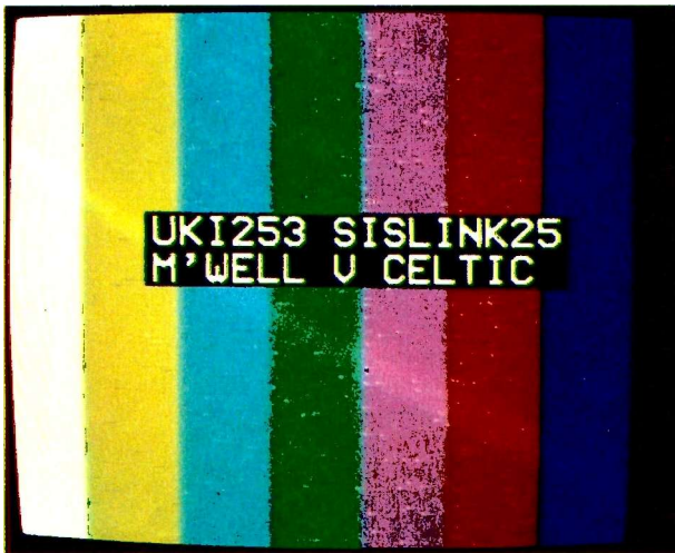
SISlink identification prior to Scottish League football via Eutelsat II F2 at 10°E. The 11.163GHz horizontal signal was received by Dean Rogers, London SE2 on January 10th.
