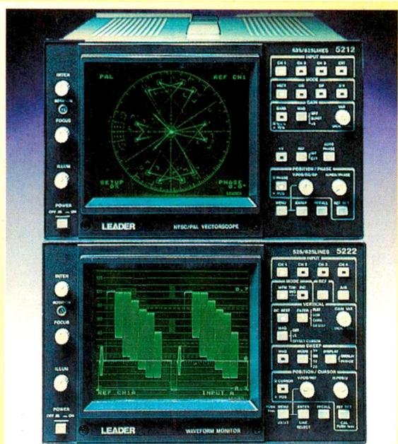
Two precision video monitors in the Leader 5000 range are now available from TTI. The 5212 vectorscope and 5222 waveform monitor offer multi-channel inputs for both composite and component signals, with automatic PAL/NTSC selection. Line selection with the 5222 enables BITS, VIR and teletext lines to be observed. For further information apply to Thurlby Thandar Instruments Ltd., 2 Glebe Road, Huntingdon, Cambs PE18 7DX. Tel 01480 412 451, fax 01480 450 409.
