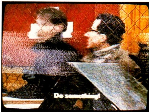
**Photo 12:** A satellite D-MAC signal makes a nice mess of UHF ch. 47 reception. In this case the outlet plate crosstalk was -30dB. Matters were made worse by a UHF signal at -10dB/mV.
