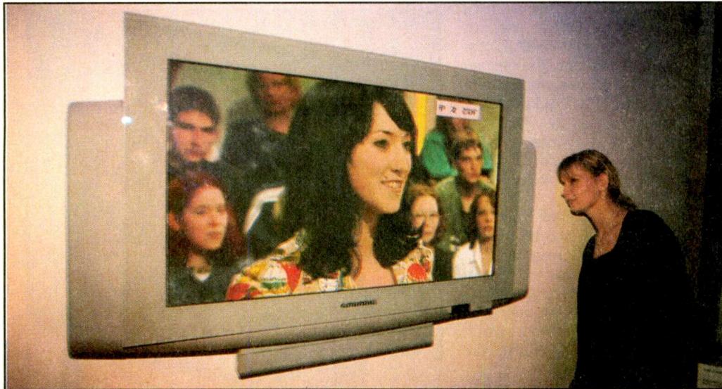
The Grundig Planatron II TV with 42in. 16:9 plasma display is just 4in. deep, with all the electronics contained within the screen section.
