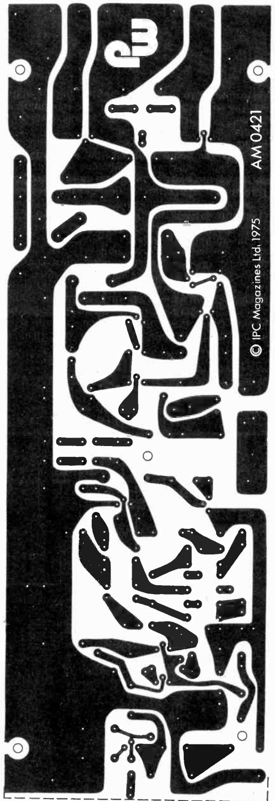
Fig. 6 and 7: Layout of the components on the amplifier board p.c.b. and printed circuit design (not to scale). The link to the right of C25 is coiled to aid high frequency stability (about ten turns).
