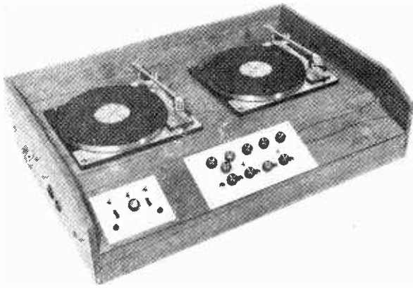
Front view of the completed Disco Unit
