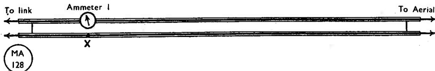
Fig. 2. The adjustment is to alter the length of feeder from point X until Ammeter 1 registers maximum reading. (See text.)
