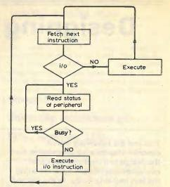
Fig. 4. Step-by-step operation of test-and-skip systems.
