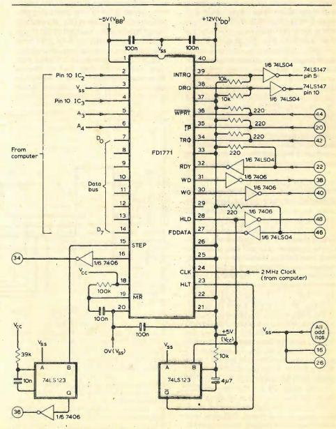
Fig. 2. Floppy-disc controller / formatter.
