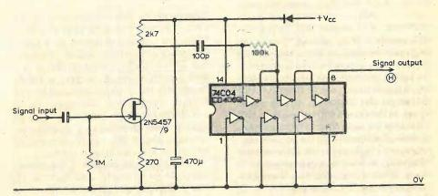
Fig. 4. Unknown-frequency input amplifier and signal conditioner.
