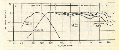
Fig. 5. Frequency response of system plotted using one-third octave pink noise signals.
