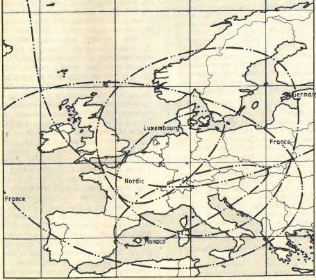
Fig. 3. Coverage area for reception on a larger antenna (1.8 to 2.0m diameter), for countries given in Figs. 1 and 2. Flux density is  $-111dB(W/m^2)$ .
