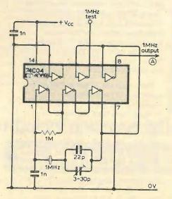
Fig. 2. Crystal oscillator, with test point output.
