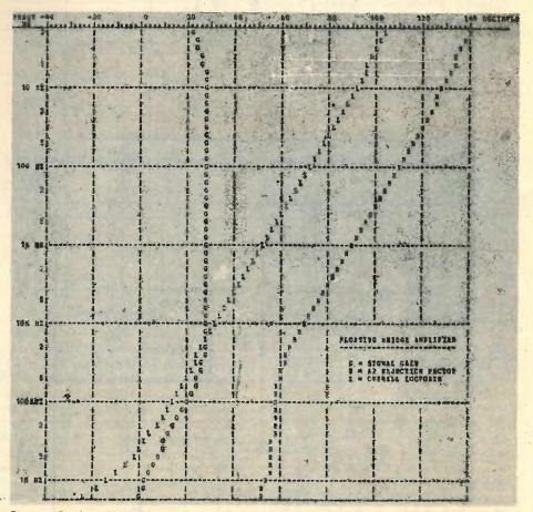
Fig. 17. Predicted performance of the amplifier, showing open-loop and closed-loop gain of  $A_1$ , and rejection factor of  $A_1$ , to distortion in  $A_2$ . Rejection factor is very high, showing that  $A_2$  can indeed be of very poor quality without affecting output.
