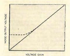
Fig. 3. Dotted line shows gain variation given by circuit of Fig. 2, where residual noise from amplifier B is predominant at low gain settings.
