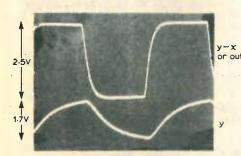
Fig. 19. Response of the 12 volt version to a 3kHz square wave input. Upper trace shows the 30kHz cutoff due to  $C_2$  in Fig. 15. Lower trace is the output of the poor quality amplifier.  $A_2$  showing cutoff at about 5kHz. Note that the output, y-x, is decoupled from the  $A_2$  output, y.
