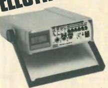
8050A 4 1/2 Digit LCD DMM with true RMS on AC volts and current DC volts 200mV-1KV, 10µV resolution AC volts. 200mV-750V, 10µV resolution. DC/AC current 200µA-2A, 0.01µA resolution resistance 200Ω-20ΜΩ, 0.01Ω resolution. Also reads dB direct referenced to 16 stored impedances. Conductance ranges 2mS and 200nS. £199 mains model £239 mains battery.
