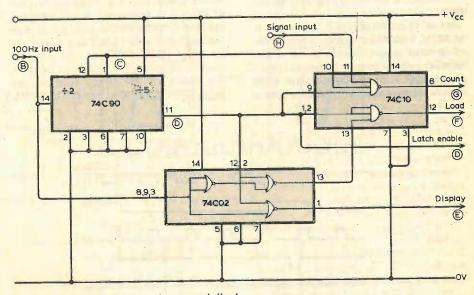
Fig. 5. Logic circuit to control gate and display.
