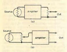
Fig. 1. Two small gain controls which do not fulfil both main requirements. Circuit (a) gives low noise, but will overload at low gain settings, while (b) introduces additional noise.
