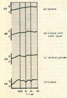
Fig. 3. Frequency response of four different cabinet shapes.
