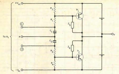
Fig. 13. Simple design for  $A_2$  — cutting all corners because distortion in this amplifier does not affect the output. So that y = -x. Gain should be about — 1 and is  $Z_{1_6}/R_1 = Z_6/R_2$ . At high frequencies, the gain must fall and so a capacitor is included in each of  $Z_5$  and  $Z_6$ . Components  $C_1$ ,  $C_2$ ,  $R_1$  and  $R_2$  are needed for  $A_1$  also and so serve a double purpose.
