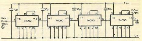
Fig. 3. Divider chain provides 100Hz for gate control.
