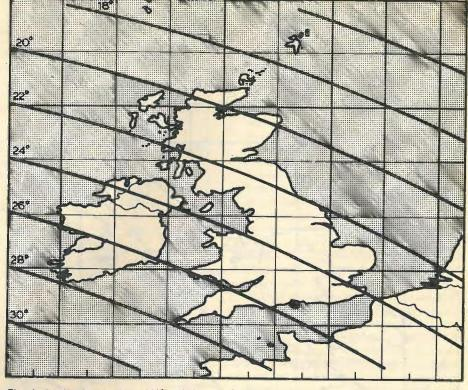
Fig. 4. Angle of elevation of UK satellite at 31\*W.
