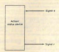
Fig. 6. Terminal characteristics of action / status devices. Signal a means that a 0 to 1 signal transition on the action terminal activates the device. No activation is possible when signal r=0. Signal r indicates the availability (r=1) or unavailability (r=0) of the device.
