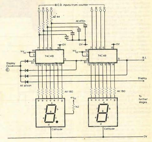
Fig. 8. Two sections of count and display circuit.
