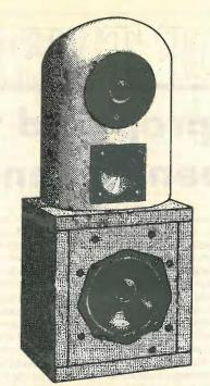
Fig. 4. Author's prototype. Clay enclosure on top contains mid and high-frequency units, while wooden bass enclosure is for B110. Single sub-woofer is not shown.
