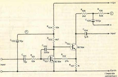
Fig. 18. Practical circuit for a ''change of origin'' for the 12 volt amplifier allows earth to be connected to the negative power rail. If a positive earth is required, use BC212 for  $Tr_{101}$  and  $Tr_{102}$  and replace point C by point D, so that a ''mirror image'' may be built.
