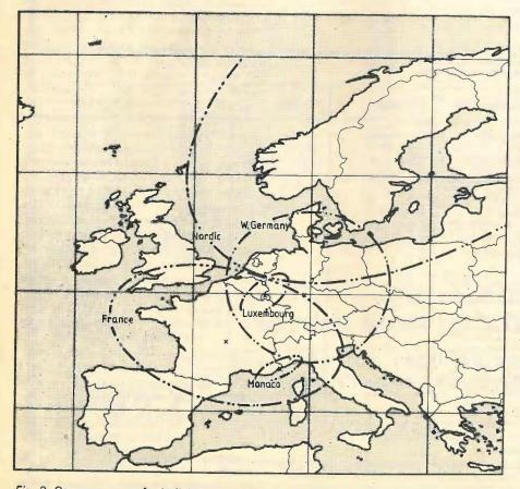
Fig. 2. Coverage areas for individual reception in W. Germany, France, Luxembourg, Monaco and the Nordic countries. Flux density is -103dB(W/m<sup>2</sup>).
