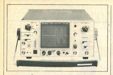
the cabinet. The MS-1650 incorporates a 118×98mm c.r.t., weighs only 9kg, measures 284×138×400mm, and costs £1440 with a two year guarantee. House of Instruments, 34/36 High St, Saffron Walden, Essex CB10 IEP. WW304
