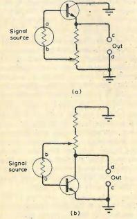
Fig. 5. Single transistor equivalent to Fig. 4, neglecting d.c. conditions. Rearrangement in (b) shows circuit to be easily recognizable. On replacing the op. amp. in Fig. 4 by a transistor, the circuit of Fig. 5(a) is obtained. Though the collector would in practice be taken to a positive supply line, it is here shown as earthed, for in the present context we are concerned only with a.c. aspects and it is best to omit irrelevant details.
