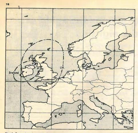
Fig. 1. Examples of coverage areas for individual reception in the UK and Ireland. Flux density is  $-103 dB(W/m^2)$ .
