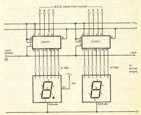
Fig. 9. Decoder and display using CD4511 latched decoder i.c.
