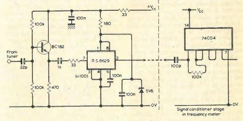
Fig. 14. Divide-by-100 prescaler for use with f.m. tuner.
