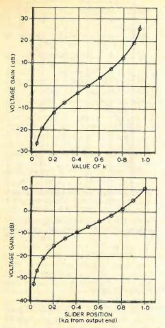
Fig. 8. Gain variation of Fig. 6(b) circuit is at (a). Measured performance of equivalent op. amp. circuit of Fig. 7 is shown at (b).
