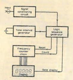
Fig. 1. General arrangement of frequency meter.
