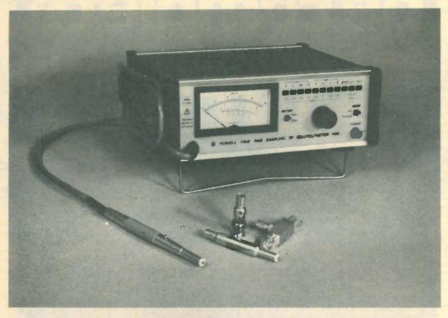
The TM8 is a new autoranging analogue true r.m.s. millivoltmeter with a specified operating range of 10kHz to 1GHz and useful indications up to 1.5GHz. It measures r.f. voltage from 1mV to 3V (or 300V using the 100:1 precision divider) and also has a logarithmic range which spans four decades – useful in setting-up tuned circuits.
