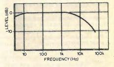
Fig. 21. Signal response of the A<sub>2</sub> amplifier as a function of frequency.
