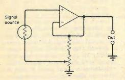
Fig. 4. Simple feedback gain control.
