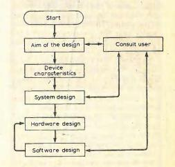
Fig. 2. Chart showing the successive steps in the design process.
