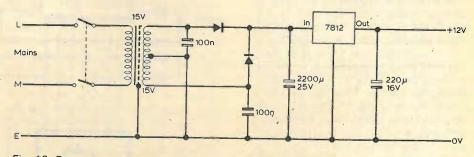
Fig. 12. Power supply circuit.
