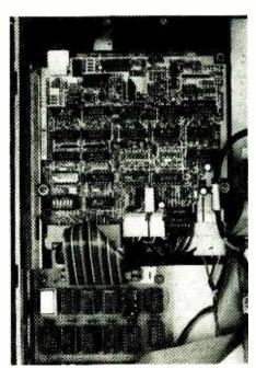
Wire-wrapped disc interface board bottom, and the disc-drive main circuit board.
