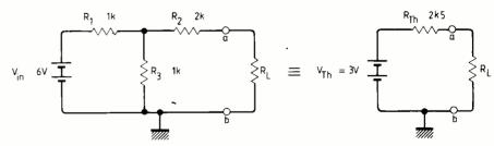
Fig. 3. Making use of the Thévenin theorem; both circuits have the same responses at the output terminals a-b.
