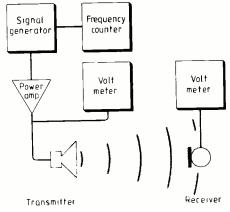
Fig. 4. Minimum instrumentation is a signal generator and suitable power amplifier, a frequency counter and a means of monitoring the transmitter drive level and receiver output voltage.
