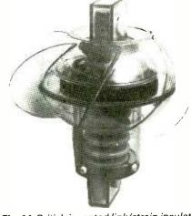
Fig. 14. British invented link/strain insulator assembly with protective shrouding. Wind-driven rotating outer dome expels water by centrifugal action. (P. F. Barber, Scarborough.)
