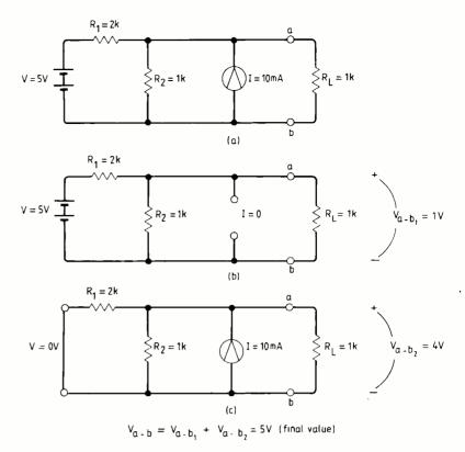
Fig. 6. Using superposition with a current and voltage source. Original circuit (a), circuit with current source open (b), and circuit with voltage source shorted (c).
