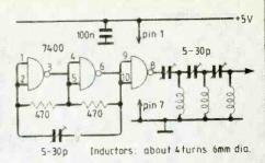
Electrically the comb generator is just an oscillator. But where normally we try to get a clean signal and suppress the harmonics here we try to produce as many as possible. We make a high pass filter by feeding the output through two or three (or more) small capacitors is series with inductors. Choose a convenient frequency for the oscillator (e.g. 10, 20, 25 or 50MHz) and fiddle both the capacitors and inductors while watching the result on the screen.
