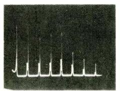
The same linearity correction should be effective on more than one band. This shows a u.h.f. display from 500 to 850MHz with 50MHz spacing.
