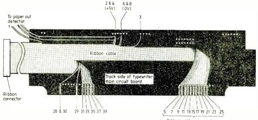
Fig. 4. 40-way ribbon cable connects the interface to the underside of the typewriter main circuit board. Alternate wires in the ribbon are connected to +5 or to 0V either at the interface end or the typewriter end. This helps to prevent crosstalk between the signal wires.
