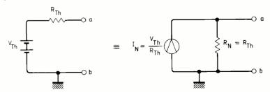
Fig. 4. Finding the Norton circuit from the Thévenin circuit.
