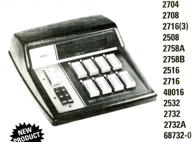
Checks, Programs, Compares up to 8 devices simultaneously
