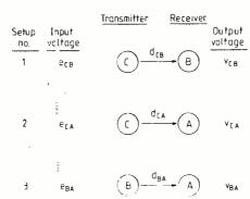
**Fig. 2.** Schematic three transducer reciprocity calibration. Drive voltage  $e_{CB}$  is applied to transducer C, which transmits to transducer B, at a distance  $d_{CB}$ , giving an output voltage  $v_{CB}$ . Test is repeated with C transmitting to A and B transmitting to A.
