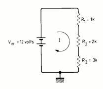
Fig. 1. Voltage divider consists of a voltage source and series resistors. (Positive current notation is used in this article.)
