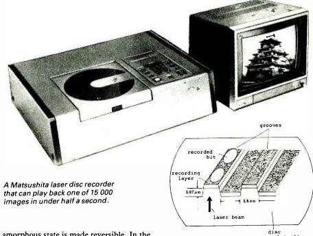
amorphous state is made reversible. In the record process the high-reflectivity crystal-line phase is converted to a low-reflectivity amorphous state; during erasure, the opposite occurs. Two semiconductor lasers are used — a 0.83µm 8mW device for recording and playback and a 0.78µm 10mW type for erasure — with a common optical system.
