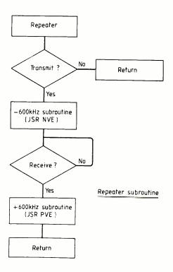
located between 1879 and 187F and uses the subroutine between 1880 and 188A to test the p.t.t. line. When the transceiver is set up to receive and has just shifted - 600kHz, another loop is entered to test for receive and reverse repeater mode (see flow chart).
