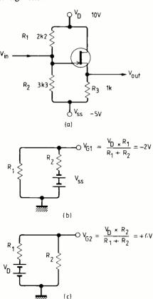
**Fig. 5.** Using superposition to find the dc bias on the gate of a j-fet amplifier. Original circuit (a), determining the effect of  $V_{SS}$  (b), and determining the effect of  $V_D$  (c).
