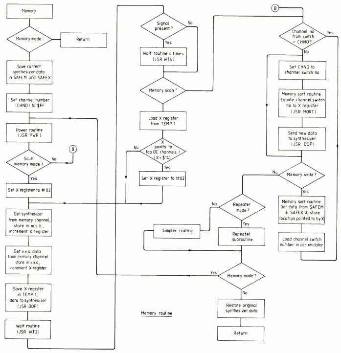
controlled crystal oscillator in 100Hz steps up to 9.9kHz. If a particular memory frequency is in use the set will wait for a period determined by the number of time that the outine at 191D is called using code between 1A94 and 1AA2. The current program calls the routine at 191D four times.
