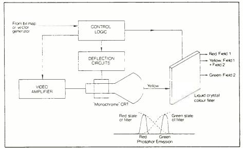
and green. In any field, information written on the screen appears in the colour selected by the electronic switch. Each colour is repeated at 60Hz, requiring the two-field system to run at 120Hz. This field-sequential system provides all possible mixtures of the two primary colours emitted by the phosphor and research is continuing to extend the concept to three fields to produce the full colour spectrum.
