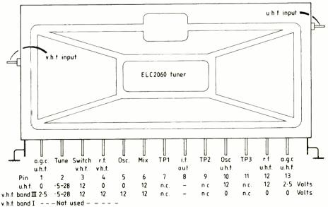
Connection details for the Philips tuner. Other tuners may be equally suitable.
