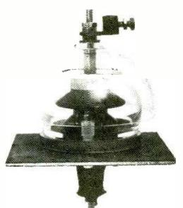
Fig. 13. Recently-developed British feedthrough assembly with dual-domed protective mantle. Moisture is expelled from domes by air blower. (By P. F. Barber, Scarborough.)
