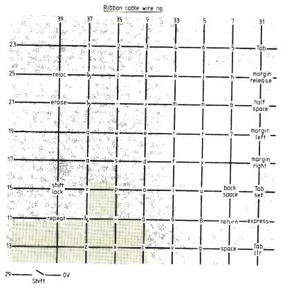
Fig. 1. Typewriter keyboard matrix: columns are each pulsed low in turn and pressing a key connects a column to a row. For clarity, diagram shows lower-case characters only.
