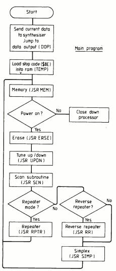
Eprom starts at 1800 hexadecimal and software breaks down into these main routines. Erase and up/down routines were covered in the April issue
