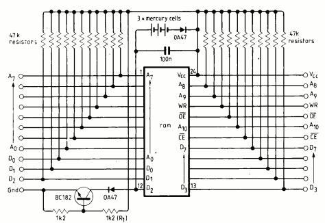
ule from external circuitry when the external supply is switched off, a transistor switch is placed in the GND line. The presence of an external supply turns the transistor 'on' and its absence turns it 'off'. The OA47 diode in series with the transistor prevents the mercury cells from discharging through R1 and the transistor's base-collector diode.
