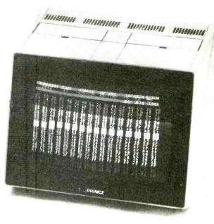
The new microprocessor controlled EP8000 Emulator Programmer will program and emulate all EPROMs up to 8k x 8 sizes, and can be extended to program other devices such as 16k x 8 EPROMs, Bipolar PROMs, single chip microprocessors with external modules.
