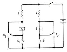
This arrangement cannot act like a buzzer, because of the toggle action. Thus relay A cannot cancel its instruction to relay B at once, but instead its changeover contact must move right across its gap. Output can be taken from a further contact. Frequency is 3-10Hz, depending on obvious factors.
