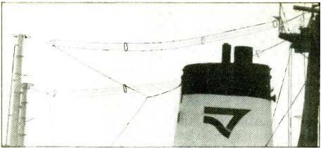
Fig. 4. Hard-to-find classic French all-wire sausage aerials with high top capacitance, well sited on available structures. ('Dumont d'Orville,' French flag, b.1977, 23910 g.r.t. photographed at Cr. Couronne, 1983.)
