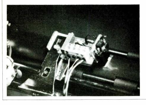
Test the connections to the typewriter by shorting out rows and columns at the connector on the end of the ribbon. Check by referring to Fig. 1 that the typewriter prints the correct character.
