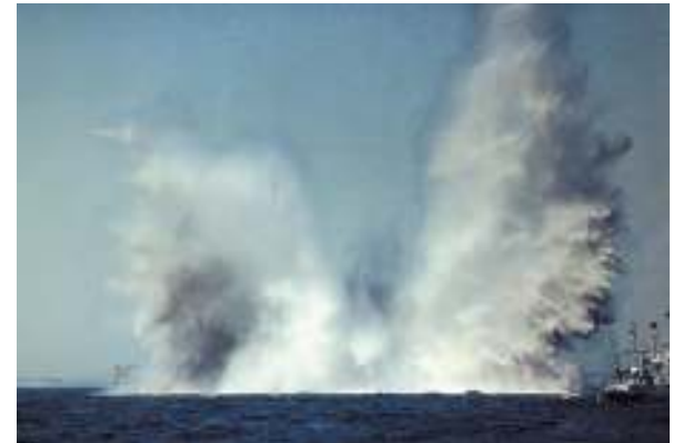
Submarine shock test of a vessel of the SM 343 class as proof of the quality of the joint platforms SM 343/MJ 332
