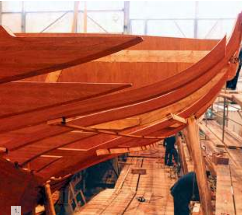
(1.) Craftsmanship that can no longer be found anywhere: traditional solid wood frame construction. (2.) You can tell just by looking: the hull is designed for extremely high speeds.
